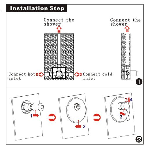
**\*** Read the Installation Fig and confirm the installing position.
